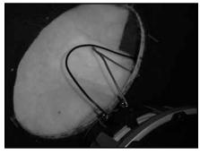
**STEP 20** Attach the proper speaker wires to the woofer's terminal.
